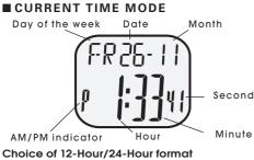
The time display format in either 12-hour indication or 24-hour indication can be selected alternately by pressing Button B. Under the 12-hour indication format, AM/PM indicator appears on the FR 56-11
