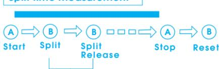
\* Measurement and release of split time can be repeated by pressing button "B".
